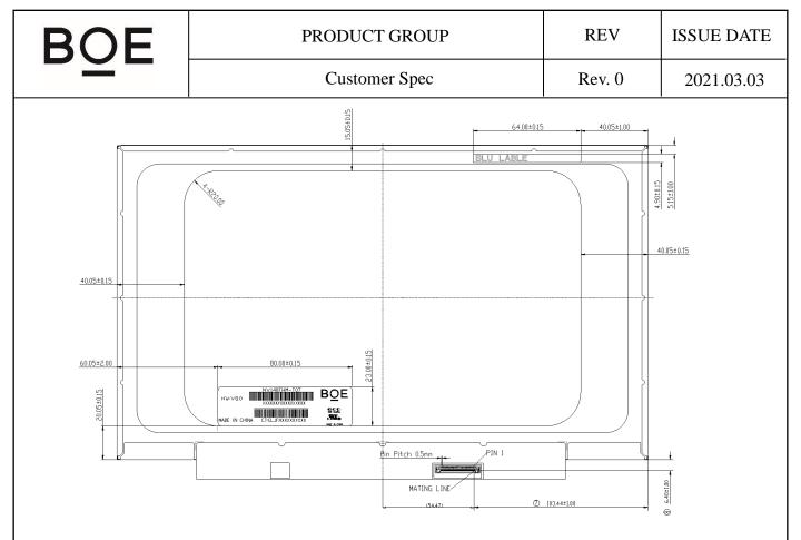
Figure 26. TFT-LCD Module Outline Dimensions (Rear view)
