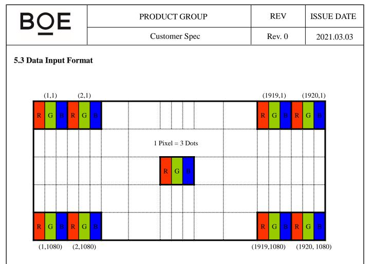
Figure 13. Display Position of Input Data (V-H)
