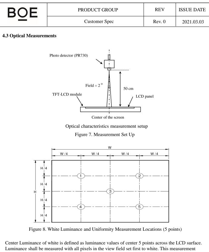
shall be taken at the locations shown in Figure 7 for a total of the measurements per display.
