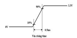
Figure 4. Inrush Measure Condition
